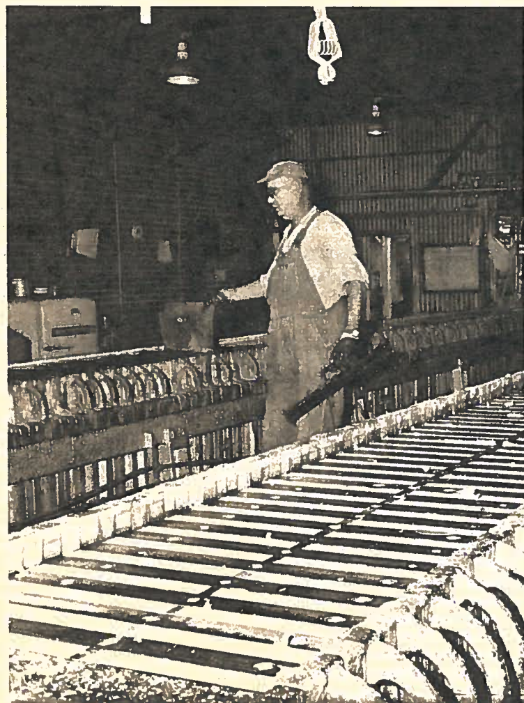
Wax is molded into slabs after refining. Molten wax flows into molds at 200 degrees.
