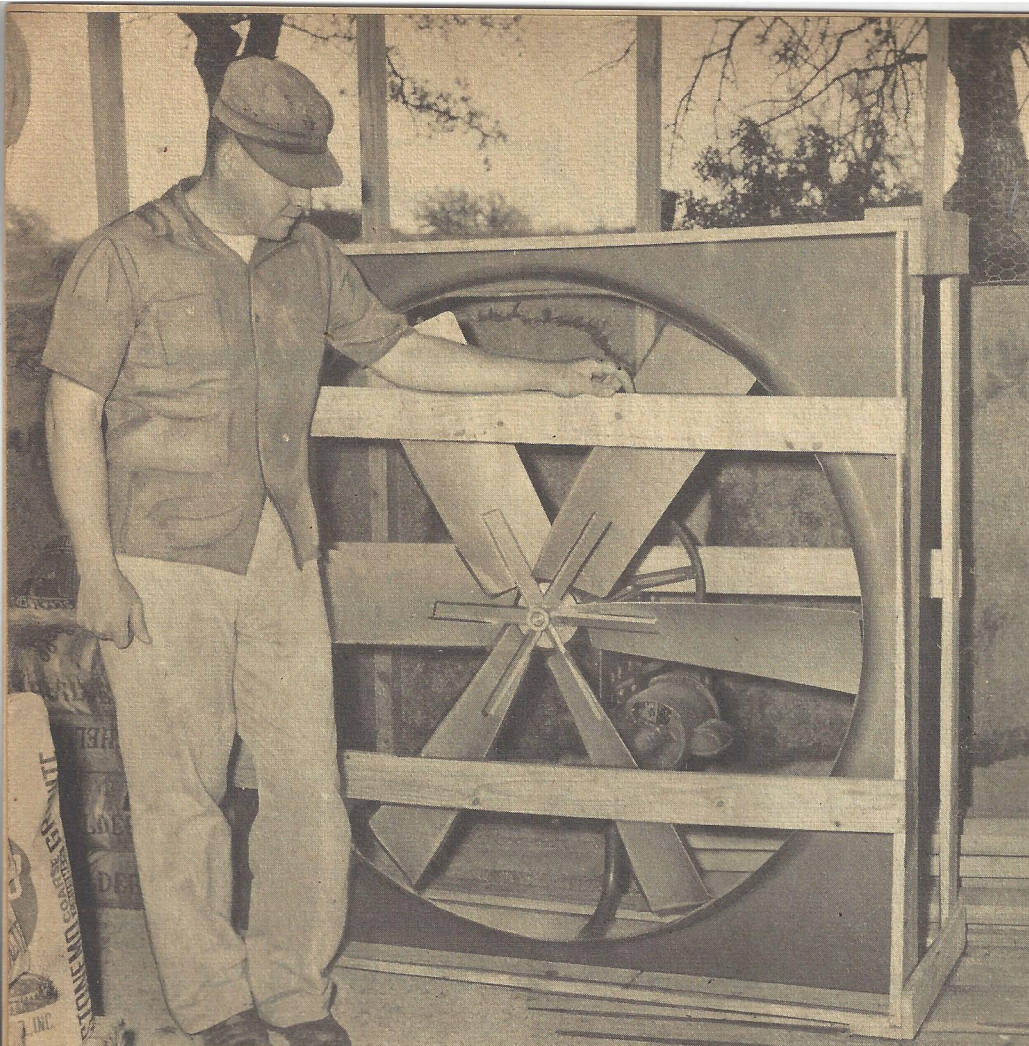
Two 4-foot fans will cool Bland Harper, Jr.'s laying house. Air temperature will be reduced 10 to 15 degrees on hot days to help hens maintain high production.
