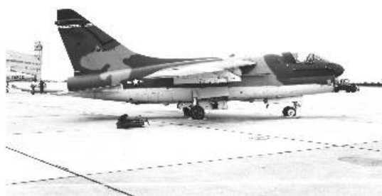
LTV A-7D (S/N 68-8224, the 10th A-7D built) at Eglin Air Force Base, Fla. Note the Navy-style refuel probe just behind the nose below the cockpit. (U.S. Air Force photo)
