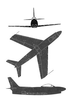
The F-86D is a single-seat interceptor developed from the F-86A Sabre. Minor design changes have given the D higher speed, highaltitude intercept, and all-weather capability. A pointed nose radome and larger aft fuselage section are the main recognition differences. The D's minor modifications include a "flying-tail-type" horizontal stabilizer, a "clamshell-type" canopy, and a more powerful engine.
