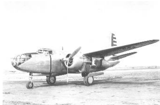
Douglas A-20. Note the turbosupercharger inlet on the outboard aft engine nacelle. (U.S. Air Force photo)
